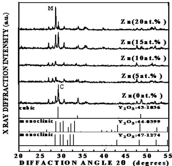
Fig. 1: X-ray diffraction patterns of Zn co-doped  $\text{Y}_2\text{O}_3$ -ZnO:Mn thin film phosphor prepared at various concentration of Zn deposited at  $600^\circ\text{C}$  and annealed at  $1020^\circ\text{C}$
