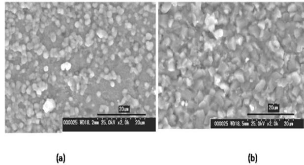
Fig. 2: SEM image of (a)  $\text{Y}_2\text{O}_3$ :Mn and (b) Zn co-doped (20at%)  $\text{Y}_2\text{O}_3$ :Mn thin film.
