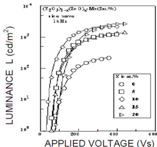
Fig. 5: L-V characteristics of Zn co-doped  $Y_2O_3-ZnO:Mn$  thin film phosphor prepared at various concentration of Zn deposited at  $600^\circ C$  and annealed at  $1020^\circ C$
