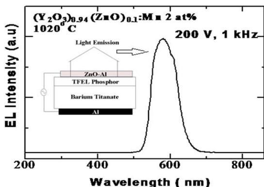
Fig. 4: EL emission spectrum of Zn co-doped (10at%)  $Y_2O_3:Mn(2at\%)$  thin film phosphor
