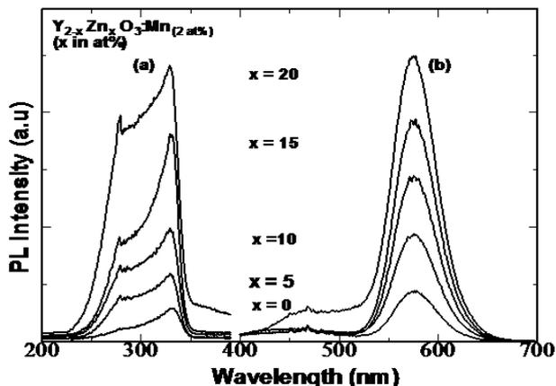
Fig. 3: Photo-luminescent excitation and emission spectra of  $Y_2O_3:Mn$  co-doped with various concentration of Zn at  $600^\circ C$  and annealed at  $1020^\circ C$
