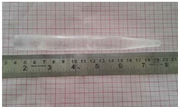
**Fig. 1(b): Photograph of Praseodymium doped KDP crystals grown by SR method**
