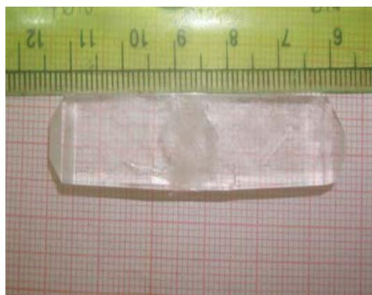
**Fig. 1(c): Photograph of Praseodymium doped KDP crystals grown by Seed Rotation technique**
