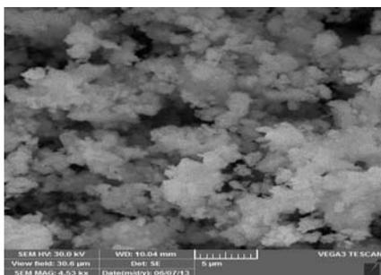
Fig.2: SEM of  $Sr_2Y_2Al_2O_8:Eu(1.5\%)$
