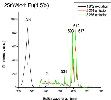
Figure-I: Excitation and emission spectrum of  $Sr_2Y_2Al_2O_8:Eu(1.5\%)$  phosphor Figure-I is the PL of  $Sr_2Y_2Al_2O_8:Eu$
