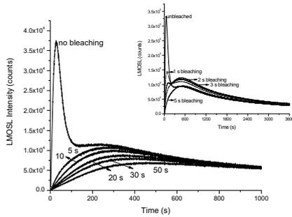
**Fig. 2c:** Effect of optical bleaching carried out using blue LEDs (90% power) on LM OSL curves. The  $\beta$  dose delivered to sample was 1.22 Gy. During LMOSL recording, the LED power was varied from 0-90% of the maximum power. For optical bleaching times from (1-5) s, the LMOSL curves are shown in the inset and the LED power was varied from 0-100% for 3600s.
