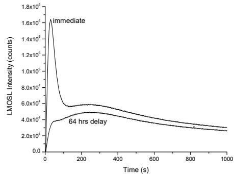
**Fig. 1c:** LM OSL curve for  $\text{CaF}_2:\text{N}$  recorded immediately as well as after 64 hours of  $\beta$  dose (1.22 Gy). Two peaks in LMOSL curve are clearly visible. The LED power was varied from 0-90% of the maximum power.
