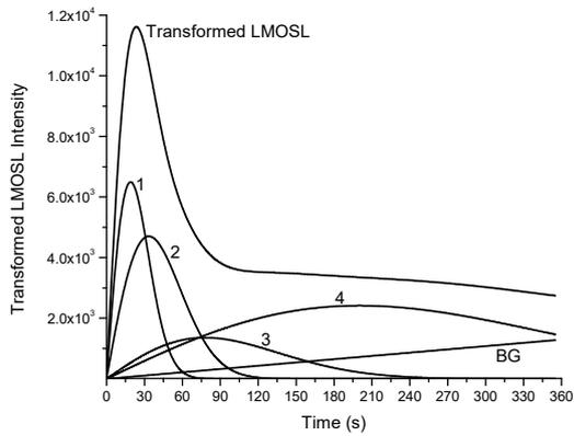
**Fig. 4c:** LMOSL components of transformed CW OSL curve corresponding to Fig. 5a. Other parameters are same as in Fig. 4a.
