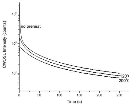
**Fig. 3b:** Effect of pre-readout annealing on CW OSL curves. The  $\beta$  dose delivered to sample was 1.22 Gy. The LED power during CWOSL recording was kept at 90% of the maximum power.
