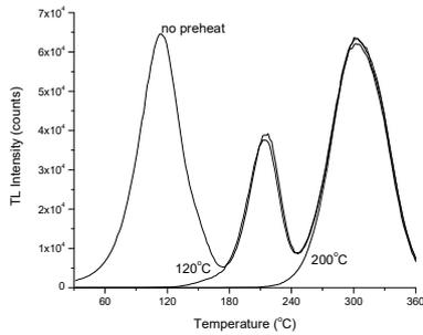
**Fig. 3a:** Effect of pre-readout thermal annealing on TL glow curves. The TL glow curves were recorded at a heating rate of  $5^\circ\text{C s}^{-1}$  and the dose delivered to the sample was 1.22 Gy.
