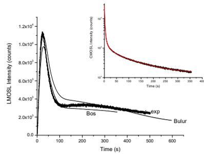
**Fig. 4a:** Transformation of CW OSL curve corresponding to Fig. 5a into LM OSL curve using Bulur and Bos techniques. The  $\beta$  dose delivered to sample was 1.22 Gy. The LED power during LMOSL recording was kept at 60% of the maximum power. The transformed LMOSL curves are also compared with the experimental curve which was recorded by varying LED power from 0-85% of the maximum power. The stimulation power and acquisition times are such that total energy incident on sample is constant.
