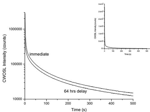
**Fig. 1b:** CW OSL curve for  $\text{CaF}_2:\text{N}$  recorded immediately as well as after 64 hours. The  $\beta$  dose of 1.22 Gy was delivered to the sample. The LED power was kept at 90% of the maximum power. The Fig. in the inset shows CWOSL curve plotted in linear scale and recorded immediately after exposure.
