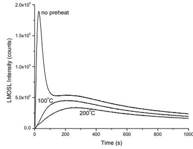
**Fig. 3c:** Effect of pre-readout annealing on LM OSL curves. The  $\beta$  dose delivered to sample was 1.22 Gy. During LMOSL recording, the LED power was varied from 0-90% of the maximum power.
