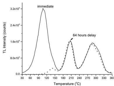
**Fig. 1a:** TL glow curve for  $\text{CaF}_2:\text{N}$  recorded immediately as well as after 64 hours. The TL glow curves were recorded at a heating rate of  $5^\circ\text{C s}^{-1}$  and a  $\beta$  dose of 1.22 Gy was delivered to the sample.
