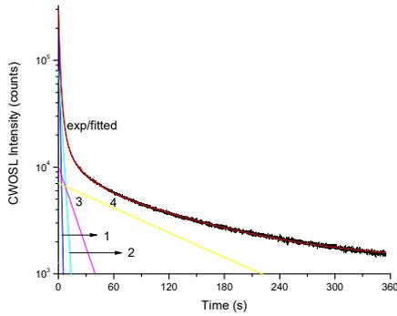
**Fig. 5a:** Fitting of experimental CW OSL curve for  $\text{CaF}_2:\text{N}$  as a sum of four first order decaying exponentials. The  $\beta$  dose of 1.22 Gy was delivered to the sample. The LED power during CWOSL recording was kept at 60% of the maximum power.
