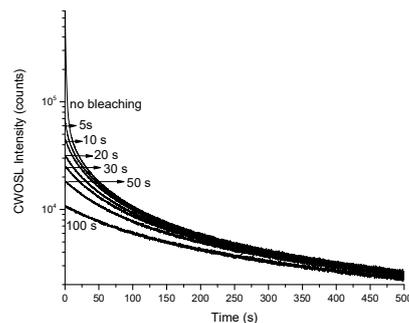
**Fig. 2b:** Effect of optical bleaching on CW OSL curves. The  $\beta$  dose delivered to sample was 1.22 Gy. The LED power was kept at 90%. The optical bleaching was carried out using blue LEDs at 90% of the maximum power.
