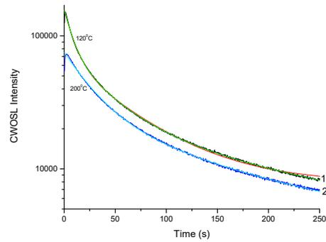
**Fig. 5c:** Fitting of experimental CW OSL curve recorded after pre-readout annealing. The  $\beta$  dose of 1.22 Gy was delivered to the sample. The LED power during CWOSL recording was kept at 90% of the maximum power. Curve no. 1 could be fitted as a sum of three first order decaying exponentials whereas the curve no. 2 could be fitted as a sum of two first order decaying exponentials.
