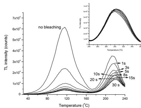
**Fig. 2a:** Effect of optical bleaching on TL glow curves. The TL glow curves were recorded at a heating rate of  $5^\circ\text{C s}^{-1}$  and the dose delivered to the sample was 1.22 Gy. Optical bleaching was carried using blue LEDs at 90% power of the maximum power. High temperature peak is unaffected by optical bleaching (inset).
