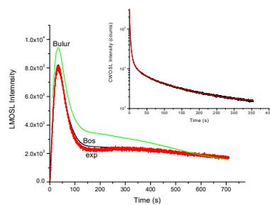
**Fig. 4b:** Transformation of CW OSL curve corresponding to Fig. 5a into LM OSL curve using Bulur and Bos techniques. The  $\beta$  dose delivered to sample was 1.22 Gy. The LED power during CWOSL recording was kept at 60% of the maximum power. The transformed LMOSL curves are also compared with the experimental curve which was recorded by varying LED power from 0-60% of the maximum power. The stimulation power and acquisition times are such that total energy incident on sample is constant.
