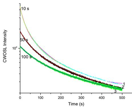
**Fig. 5b:** Fitting of experimental CW OSL curve recorded after bleaching times for 10s, 50s and 100s. The  $\beta$  dose of 1.22 Gy was delivered to the sample. The LED power during CWOSL recording was kept at 90% of the maximum power. Curve no. 1 could be fitted as a sum of three first order decaying exponentials whereas the curves no. 2 and 3 could be fitted as a sum of two first order decaying exponentials.
