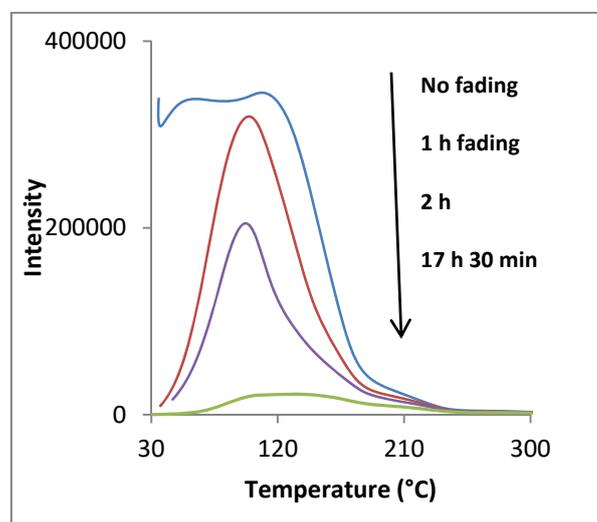
Fig.1: TL curves of the  $\text{Sr}_4\text{Al}_{14}\text{O}_{25}:\text{Eu}^{2+},\text{Nb}^{3+}$ . Excitation: Tubelight for 5 min;  $\beta=1^\circ\text{C/s}$ .
