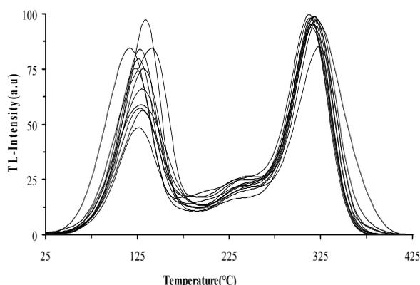
**Fig. 1:** A set of twelve glow curves of  $\beta$ -irradiated at RT (22°C) NaCl powder with a dose of 15Gy.
