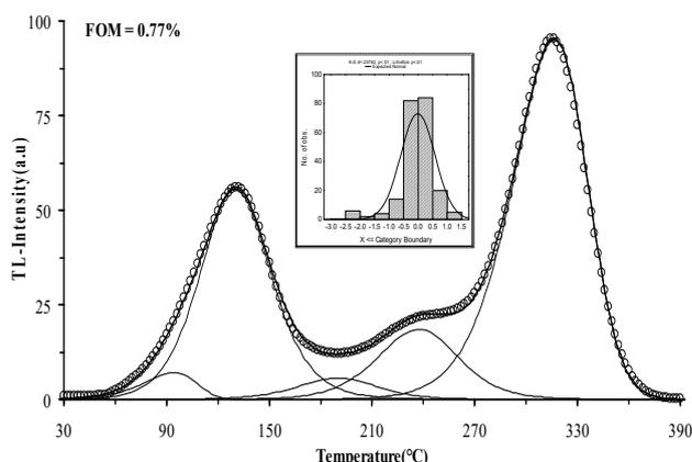
**Fig. 2:** CGCD of typical glow curves of NaCl (showing peaks). (Inset: Histogram of errors with the expected normal curve in fitting glow curve)
