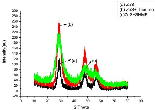
Fig 1.XRD Pattern of ZnS(uncapped and capped) nanoparticles.
