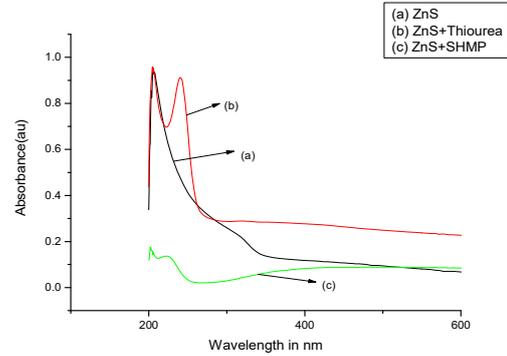
Fig2. UV-visible Absorption spectrum of ZnS(uncapped and capped)nanoparticles.
