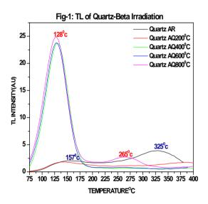
quenched from 200, 400, 600 and 800°C for an hour is interesting to note the TL peak temperature is found around 150°C and followed by another peak around during annealing the
